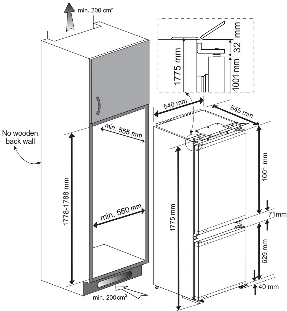
The back wall of the wooden cabinet must be left open completely to the kitchen wall in order to allow sufficient air circulation to cool down the condenser unit for energy efficiency.
